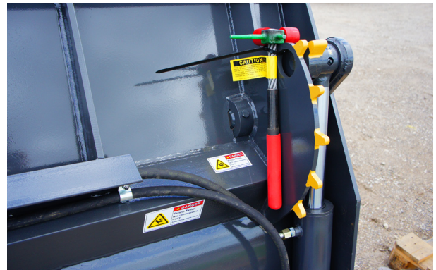
Dymax opening indicator allows operators to know general clam positioning.
