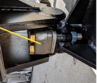
Shim adjustable lower ball joint provides oscillation when slotted retainer is installed.
