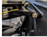
Each blade is provided with two pin retainers. All models are shipped with the fixed retainer installed.
